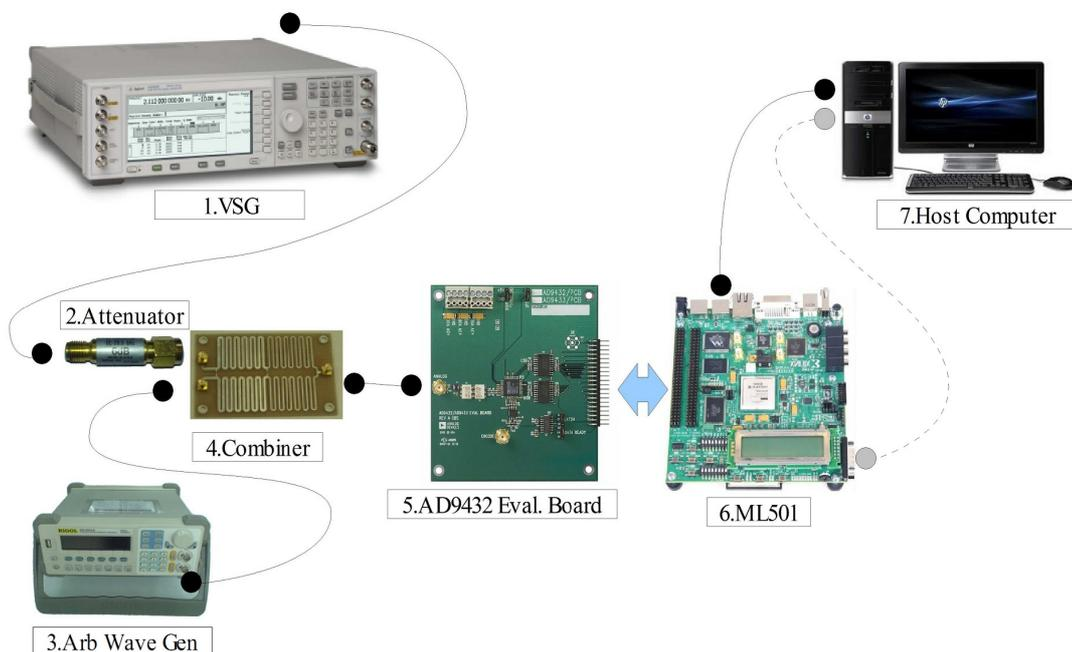
Fig. 2. Real-time hardware testbed
