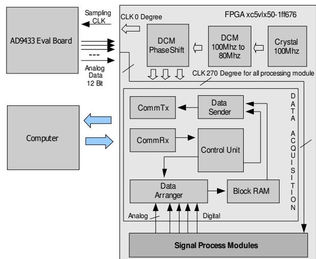
Fig. 3. Architecture overview of digital signal processing platform
