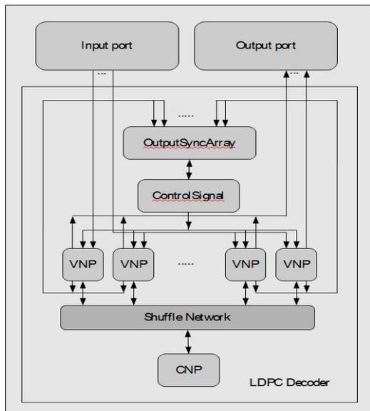
Fig. 1. Architecture of flexible LDPC decoder
