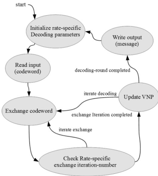
**Fig.7.**Finite State Machine of LDPC Decoder.
