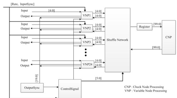
(a) Overall architecture of Scheme 1: a stage of register is added between shuffle network and CNP
