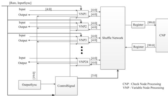
(b) Overall architecture of Scheme 2 and Scheme 3: a couple stage of registers is added between shuffle network and CNP
