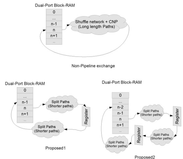
**Fig.6.** Conceptual illustration of pipelining and retiming.
