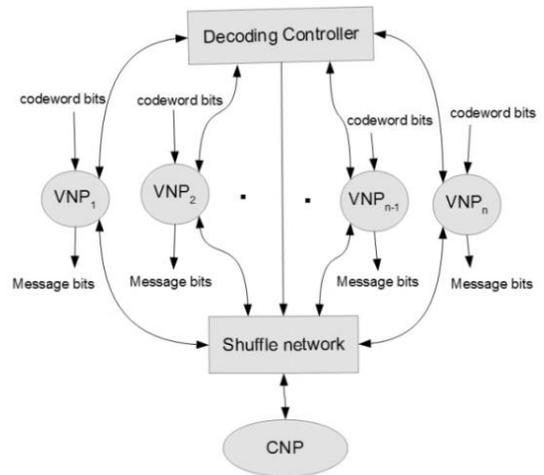
Fig.2. The architecture of flexible LDPC decoder.
