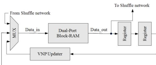
(e) Register insertion in VNP22 - VNP24 of Scheme 3. The rest of VNPs are the same as those in Scheme 2.
