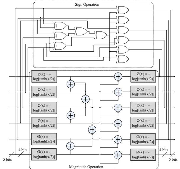
Fig.3. The architecture of CNP.
