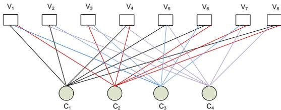
**Fig.1.** Bipartite or Tanner graph representation of an LDPC code mainly consisting of variable nodes, check nodes, and edges.
