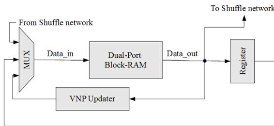
(c) Register insertion in all VNPs of Scheme 1
