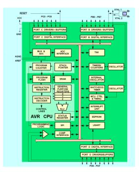
The central feature is the AVR core consisting ALU, 32 general purpose registers including three index registers, processor status register, stack pointer and program counter with instruction register and instruction decoder.
