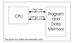
John Von Neumann's: One shared memory for instructions (program) and data with one data bus and one address bus between processor and memory. Instructions and data have to be fetched in sequential order (known as the Von Neuman Bottleneck), limiting the operation bandwidth. Its design is simpler than that of the Harvard architecture. It is mostly used to interface to external memory.
